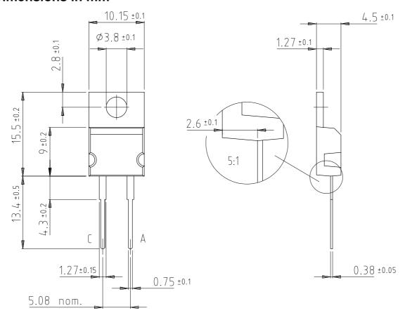
Plastic case JEDEC DO 220 Cathode connected with metallic surface
